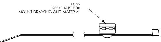
DELIVERY CONDITION: CABLE TIE HEAD COULD BE AT THE LEFT OR RIGHT SIDE OF EDGE CLIP
