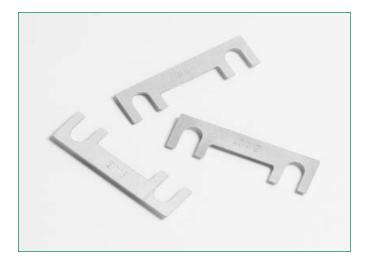
Non-housed fuse strips for Diesel vehicles. Current rating 25A - 150A, 36 VDC. 90° fork type lugs.
