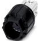
QUICKON nut, black, 3-pos. +PE, 1.0 mm<sup>2</sup> ... 2.5 mm<sup>2</sup> / 630 V / 20 A, for cables with diameters of 6 mm ... 10 mm.
