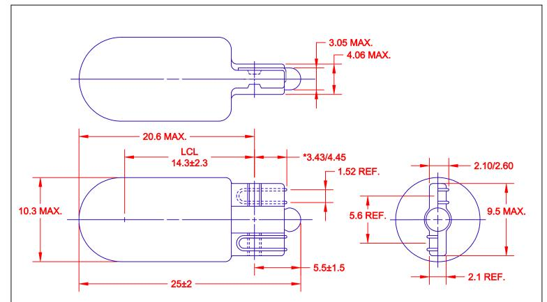
\*TO BE MEASURED ON LONGEST SIDE ONLY WITH THE WIRE IN INTIMATE CONTACT WITH THE BOTTOM OF THE GLASS WEDGE.
