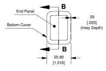
**SECTION B-B** 2.20 (Inside of Bottom Cover) 1.0861 (PCB dist from inner wall)
