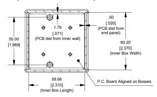
Enclosures can be Factory Modified (Milling, Drilling, Printing etc.) Solid models of this enclosure available in STEP or IGES.
