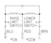
MOTOR CIRCUIT 120V, 50/60 HZ \* ROTATION AS VIEWED FROM MOTOR END MOTOR SPEED: SEE CHART  $\pi$  if ganged units are used in a system that ordinarily
