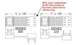
$\label{eq:approx} \begin{array}{l} \mbox{``A}^{*} = (\text{No. of Conductors x } 0.050 \; [1.27]) + 0.095 \; [2.41] \\ \mbox{``B}^{*} = (\text{No. of Conductors -1}) \times 0.050 \; [1.27] \\ \mbox{``E}^{*} = (\text{No. of Conductors +1}) \times 0.050 \; [1.27] \\ \mbox{``F}^{*} = (\text{No. of Conductors -1}) \times 0.050 \; [1.27] \end{array}$
