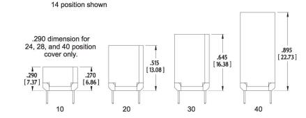
ALL DIMENSIONS: INCHES [MILLIMETERS] ALL TOLERANCES: ±0.005 [0.13] UNLESS OTHERWISE SPECIFIED FOR MATING DIP HEADER, SEE <u>DATA SHEET 12032</u> CONSULT FACTORY FOR OTHER SIZES AND CONFIGURATIONS CUSTOMIZATION: ARIES SPECIALIZES IN CUSTOM DESIGN AND PRODUCTION. SPECIAL MATERIALS, PLATINGS, SIZES, AND CONFIGURATIONS CAN BE FURNISHED, DEPENDING ON QUANTITY.
