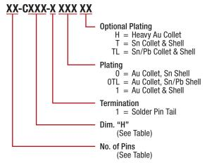
**ALL DIMENSIONS: INCHES [MILLIMETERS]** ALL TOLERANCES: ±0.005 [0.13] UNLESS OTHERWISE SPECIFIED FOR COLLECT SOCKETS W/SURFACE MOUNT PINS, SEE DATA SHEET 12023 FOR COLLET SOCKET w/WIRE WRAP PINS, SEE DATA SHEET 12025 CONSULT FACTORY FOR OTHER SIZES AND CONFIGURATIONS
