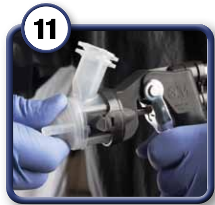
11 Re-attach the same atomizing head or when necessary replace with a new one.
