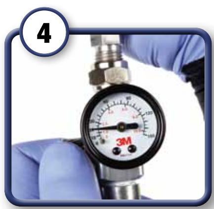
4 Set air pressure at 20 psi at full trigger (air and fluid flowing).
