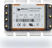
Micro example: V375C24C150BG 375 Vin, Micro, 24 Vout @ 150 W, long RoHS pins, slotted baseplate
