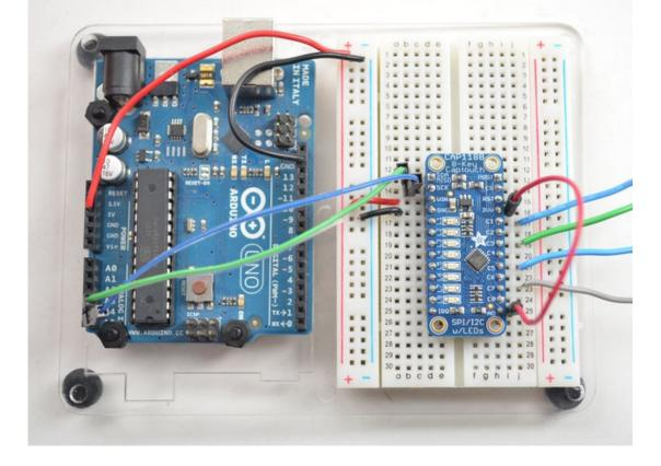
If you want to set the I2C address to a different value you'll need to connect a resistor from **AD** to ground instead of a wire to 3V. The datasheet talks about different resistor values in table 3.1 - but since the breakout board already has a 150K resistor on it, you'll need to use different values so that the parallel resistance comes out right. Here's the values you should use:
