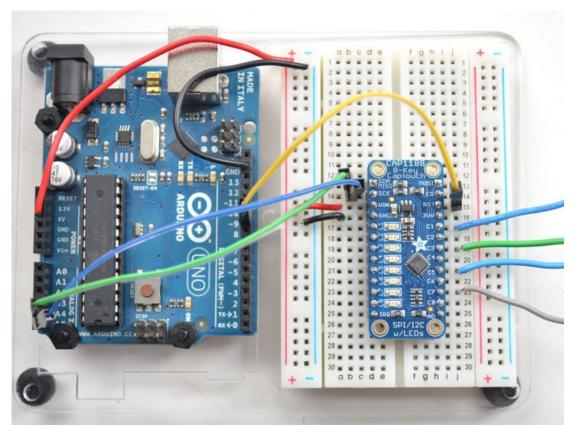
If you're using multiple sensors, or you just want to change the I2C address to something else, you can choose from 5 different options - **0x28**, **0x29** (default), **0x2A**, **0x2B**, **0x2C** and **0x2D** The I2C address are selected by connecting a resistor to the**AD** pin in the lower right: different resistors set a different address. The easiest address to set is 0x28 which is just a wire from **AD** to the **3Vo** pin.
