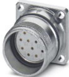
Device connector for front wall, straight, shielded: yes, Screw locking, M23, Number of positions: 17, Type of contact: Socket, Crimp connection, Radial O-ring, 4x Ø 3.2
