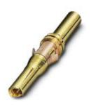
Crimp contact, turned, Contact diameter: 1 mm, Crimp range: 0.08 mm<sup>2</sup>...0.22 mm<sup>2</sup>
