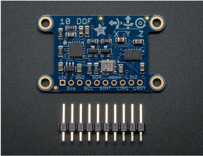
Please note that there is a small cosmetic error on the first revision of these boards (shown above). The straight X arrow for the accelerometer should be pointing in the opposite direction, towards the right. This will be fixed in the net run of these boards.
