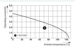
Derating diagram (6 modules in HC-B 24 housing)
