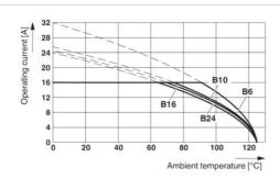
The illustration shows the derating diagram of various series B contact inserts (B6 to B24), conductor cross section 2.5 mm<sup>2</sup>
