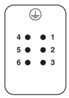
Connector pin assignment, connection side
