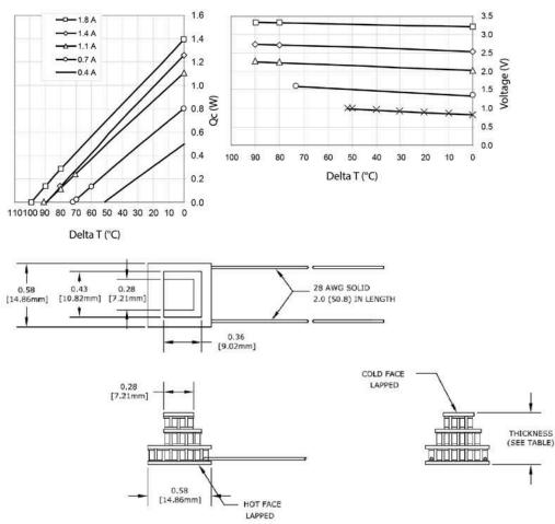
Ceramic Material: 100% (Al<sub>2</sub>O<sub>3</sub>) Solder Construction: 138°C, Bismuth Tin (BiSn)
