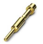
Crimp contact, turned, Single contact, contact diameter: 1 mm, crimp range: 0.5 mm<sup>2</sup> ... 1.5 mm<sup>2</sup>
