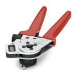
Crimping pliers for turned crimp contacts Ø 1.0 mm / Ø 1.6 mm / Ø 2 mm / Ø 3.6 mm, litz wire cross section of 0.08 mm<sup>2</sup> ... 6 mm<sup>2</sup>
