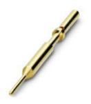
Crimp contact, turned, Contact diameter: 0.6 mm, Crimp range: 0.34 mm<sup>2</sup>...0.5 mm<sup>2</sup>
