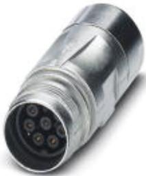
Coupler connector, straight, SPEEDCON locking, M17, Number of positions: 5+3+PE, Type of contact: Socket, Crimp connection, shielded: yes, Cable diameter: 3.5 mm...5.5 mm
