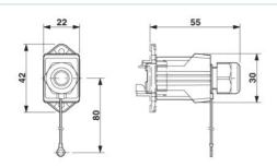
Protective cover for the Push-Pull panel mounting frame
