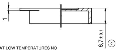
TO PREVENT DAMAGE AT LOW TEMPERATURES NO IMPACT OR EXTREM MECHANICAL LOAD SHOULD APPLIED TO THE CAP:
