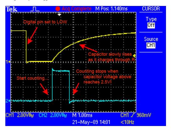
This capture from an oscilloscope shows whats happening on the digital pin (yellow). The blue line indicates when the sketch starts counting and when the couting is complete, about 1.2ms later.
