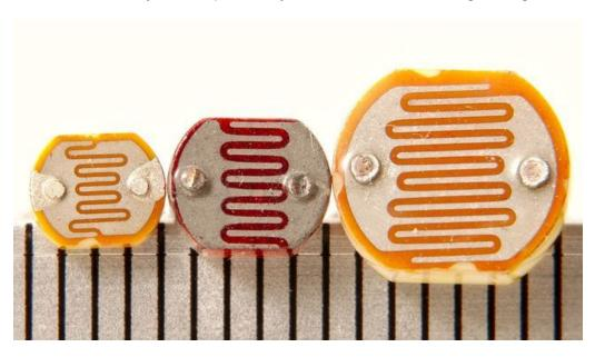
For most light-sentsitive applications like "is it light or dark out", "is there something in front of the sensor (that would block light)", "is there something interrupting a laser beam" (break-beam sensors), or "which of multiple sensors has the most light hitting it", photocells can be a good choice!
