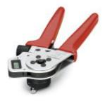
Crimping pliers for turned RC crimp contacts Ø 1 mm / Ø 1.5 mm / Ø 2 mm, litz wire cross section of 0.08 mm<sup>2</sup> ... 2.5 mm<sup>2</sup>
