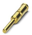
Crimp contact, turned, Contact diameter: 2 mm, Crimp range: 2.5 mm<sup>2</sup>...4 mm<sup>2</sup>
