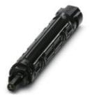
Fuse connector for protecting modules and devices in photovoltaic systems, black, SUNCLIX pin connector pattern, 1000 V/8 A, IP68 (24 h/2 m)
