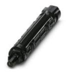
Fuse connector for protecting modules and devices in photovoltaic systems, black, SUNCLIX pin connector pattern, 1000 V/12 A, IP68 (24 h/2 m)
