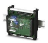
The EV-CC-AC1-M3-CBC-SER-HS charging controller with housing for DIN rail mounting is used for charging electric vehicles at 3-phase AC networks according to IEC 61851-1, Mode 3. Optimized for charging stations with permanently mounted Vehicle Connector. All charging functions and comprehensive configuration settings are already integrated.
