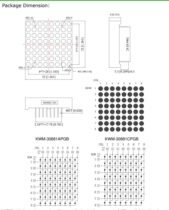
NOTES: All dimensions are in millimeters (inches) tolerance are  $\pm 0.25$ mm (0.01inch) unless otherwise noted.
