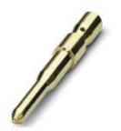
Crimp contact, leading (PE), turned, contact diameter: 1.5 mm, crimp range: 0.5 mm<sup>2</sup> ... 1 mm<sup>2</sup>
