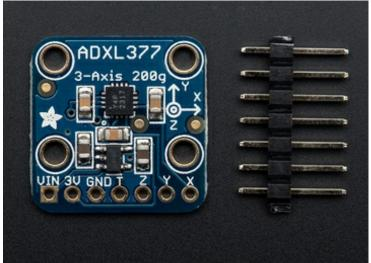
The ADXL377 can measure at least  $\pm$  200G(!) in the X, Y and Z axis. This is the sensor for measuring extreme dynamic accelerations encountered in applications such as rocketry experiments and high-impact shock measurements.
