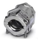
Metal screw connection with strain relief clamp, thread length: 7 mm, cable sealing area: 10 - 19 mm, clamping area: 12 - 22 mm, SW 30, screw connection: M25
