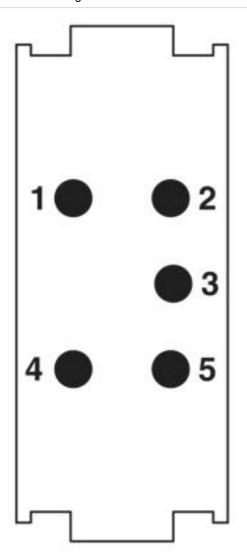
Connector pin assignment, connection side
