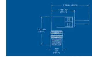
Anti-vibration coupling nuts standard.
