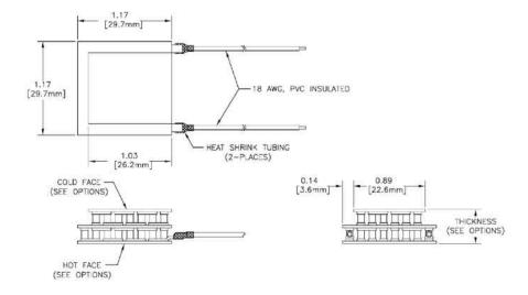
Ceramic Material: Alumina (Al<sub>2</sub>O<sub>3</sub>)
