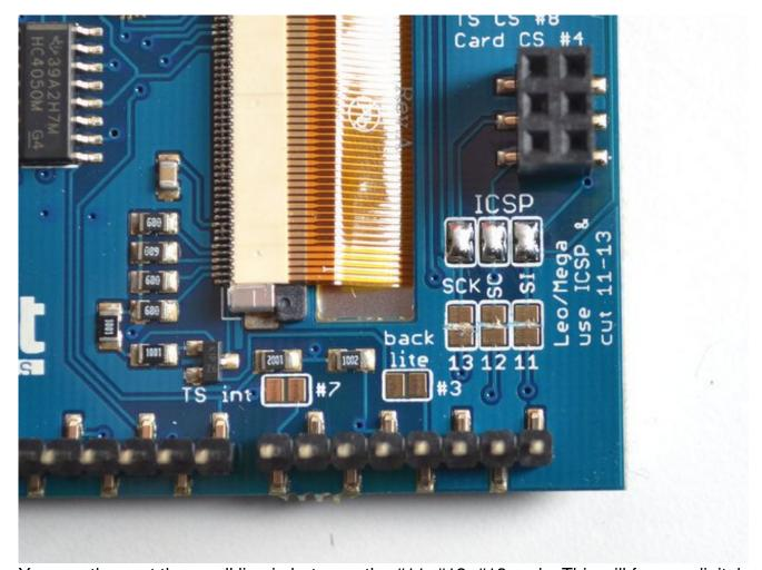
You can then cut the small line in between the #11, #12, #13 pads. This will free up digital #11, 12, and 13 for you to use on the Leo or Mega.
