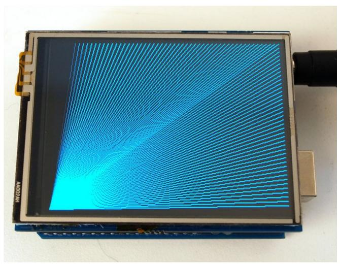
Restart the Arduino software. You should see a new **example** folder called **Adafruit\_ILI9341** and inside, an example called **graphicstest**. Upload that sketch to your Arduino! You should see a collection of graphical tests draw out on the TFT.
