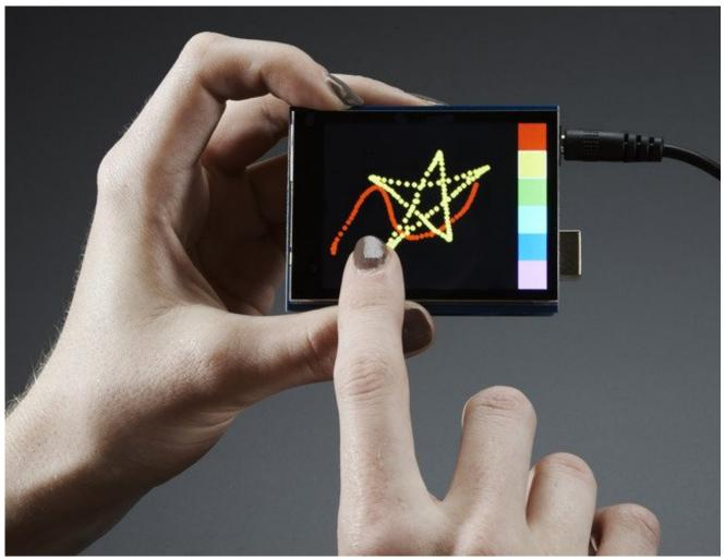
This shield uses a SPI display - its much easier to use with Mega & Leonardo than our v1 shield. We also include an SPI resistive touchscreen controller or a I2C capacitive touch screen controller so you only need one or two additional pins to add a high quality touchscreen controller. Even with all the extras, the price is lower thanks to our parts sourcing & engineering skillz!
