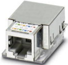
RJ45 socket insert, for the Freenet system, CAT5e, 8-pos., shielded, with cable connection (IDC fast connection), for solid wires AWG 24 ... 22
