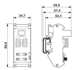
Patch panel with one RJ45 connection
