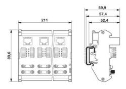
Patch panel with eight RJ45 connections
