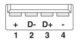
Pin assignment plug USB, type A
