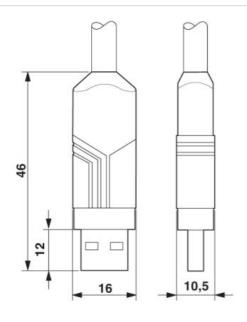
USB plug connector, type A, Standard
