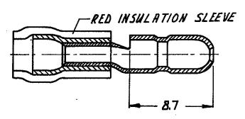
To be crimped with a SUPERCHAMP hand tool only.
