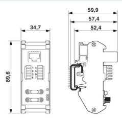
Patch panel with one RJ45 connection
