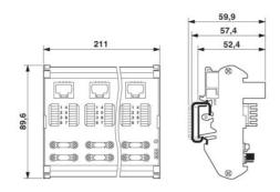
Patch panel with eight RJ45 connections
