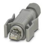
RJ45 connector, IP67, CAT5e, 8-pos., with QUICKON fast connection technology, for 1-wire and 7-wire conductors AWG 26 ... 22, for cable diameter of 5.0 mm ... 8.0 mm, TIA 568 B labeling, color: gray
