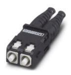
SCRJ fiber optic connector, IP20, duplex, with fast connection technology, for fiberglass multi-mode 50/125  $\mu$ m, for individual wire diameter 2.9 mm
