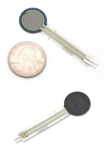
The FSR is made of 2 layers separated by a spacer. The more one presses, the more of those Active Element dots touch the semiconductor and that makes the resistance go down.
