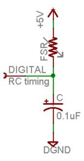
In this case, our 'bucket' is a 0.1uF ceramic capacitor. You can change the capacitor nearly any way you want but the timing values will also change. 0.1uF seems to be an OK place to start for these FSRs.
