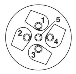
Cable connection side M12 (screw connection)
